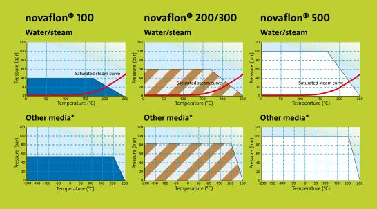
The temperature and pressure recommendations in the graphs apply to gaskets with a thickness of 2.0 mm and smooth flanges. Higher stresses are possible when thinner gaskets are used!
